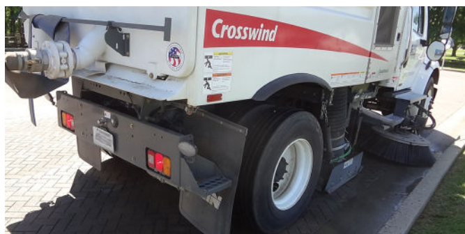
Figure 1. Typical street sweeper used to remove surface debris from large ICP areas in the spring and fall.
