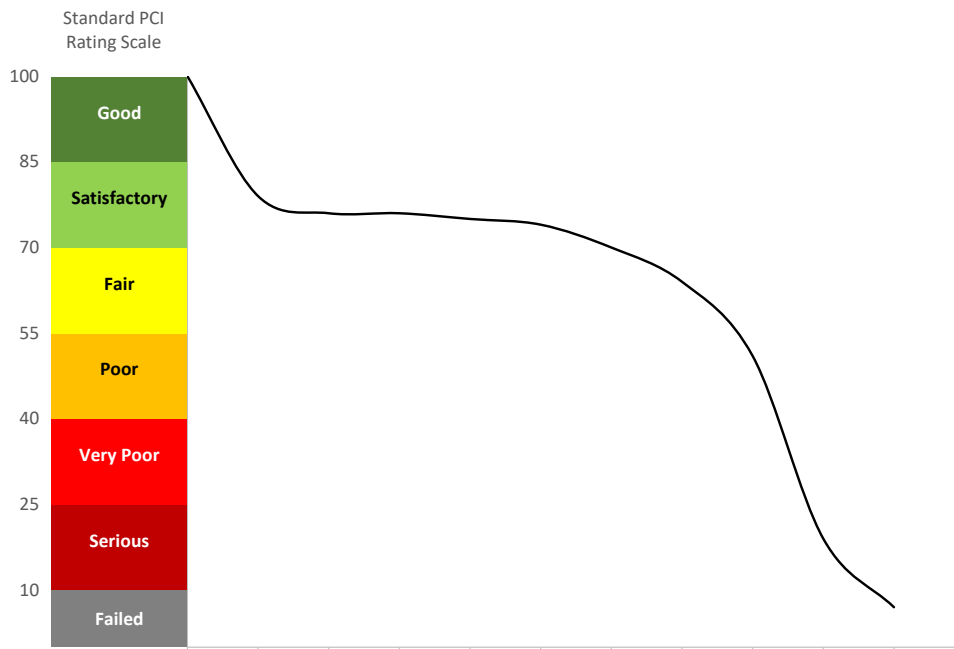
Figure 16. Pavement Condition Index Surveys can be used to predict when maintenance might be required.
