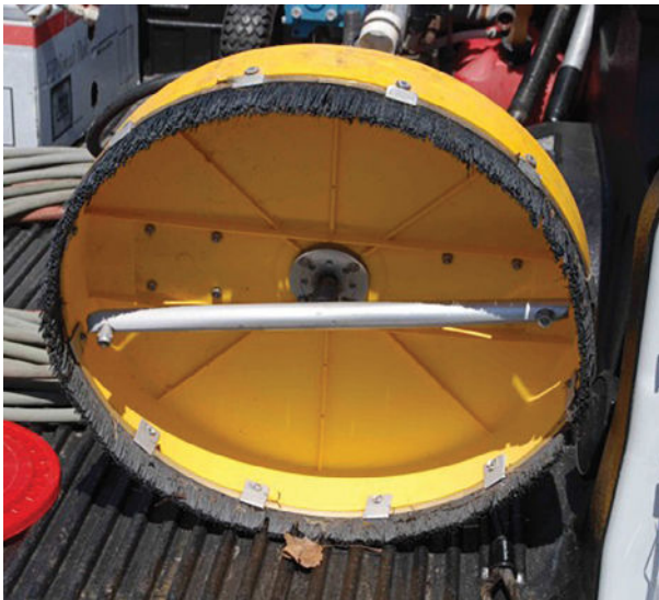
Figure 12. From the underside of the pressure washing attachment, it is possible to see the rotating pressure wand, which sprays the pavement surface.
