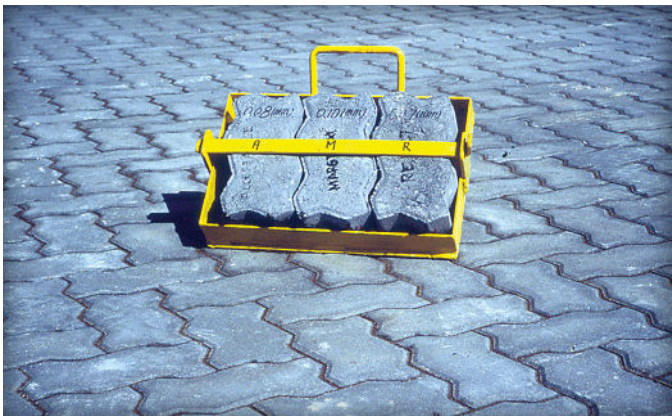
Figure 16. A simple gauge for checking dimensional tolerances on the job site.
