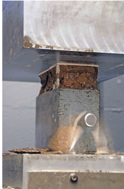
Figure 6. Left: a capped concrete paver under load in a compression testing machine; Right: a paver tested in compression; the moment it breaks is the recorded load.
