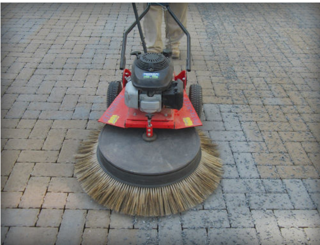
Figure 16. Rotary brushes increase cleaning efficiencies.
