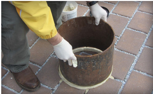
Figure 12. Steps in setting up test equipment for measuring surface infiltration using ASTM C1781.
