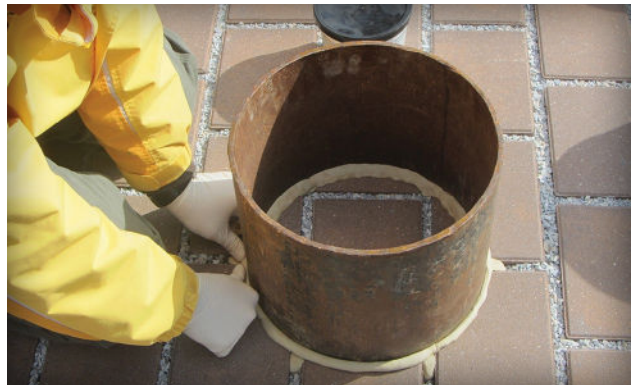
Figure 12. Steps in setting up test equipment for measuring surface infiltration using ASTM C1781.
